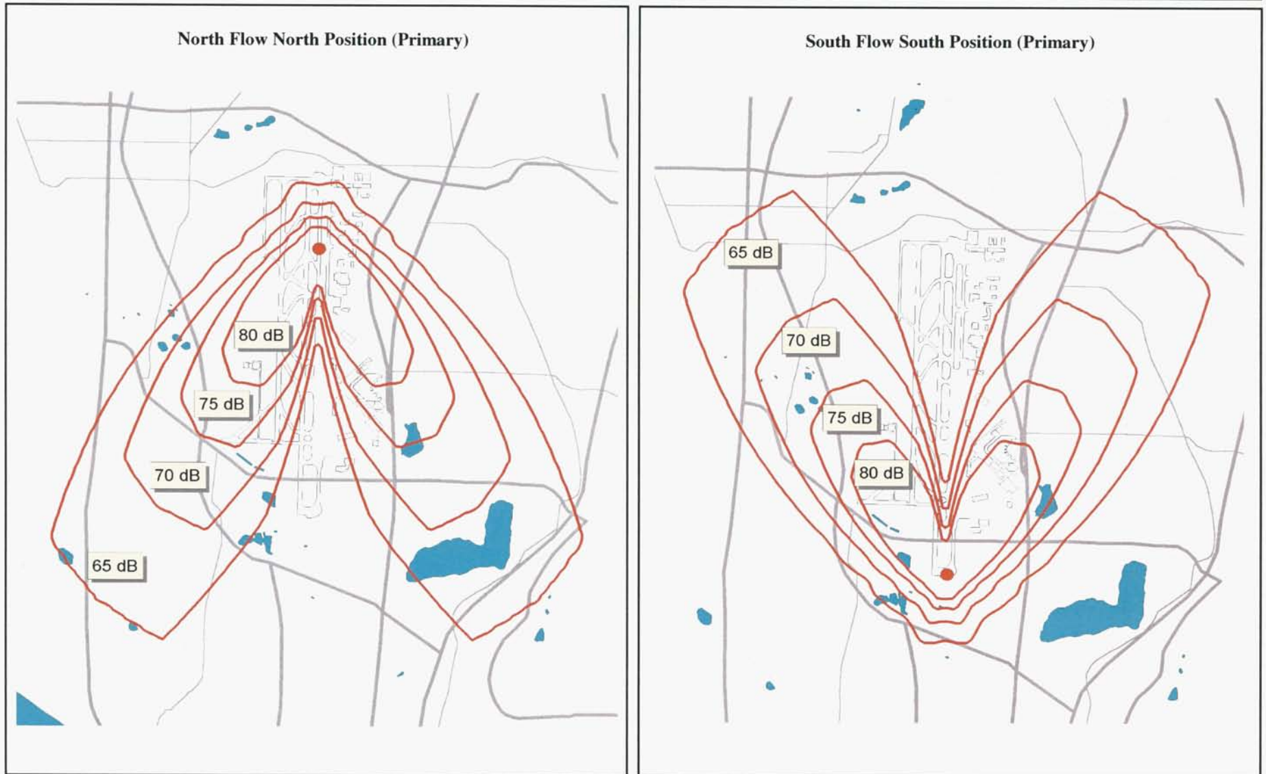
Figure E.4 Seattle Tacoma International Airport Part 150 Noise Study Example of Noise Levels for Aircraft Maintenance Run-ups A-weighted -- Full Power Run-up of B737-200
